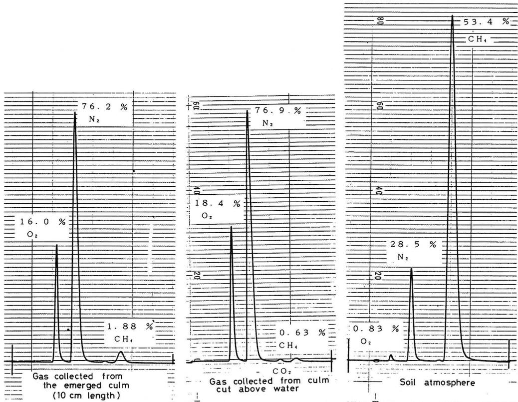
Fig. 8. Composition of gases.
