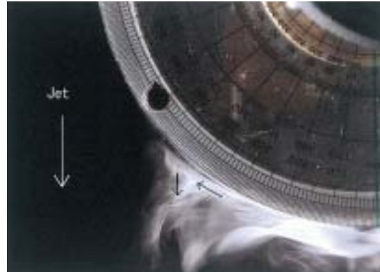
Fig. 5 Flow visualization by smoke-wire method (Measurement of separation angle)
