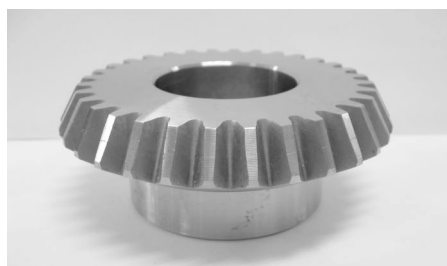
(a) Straight conical gear
