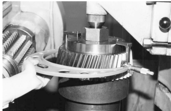
Fig.11 Cutting conical gear used for marine transmissions by table sliding taper hobbing
