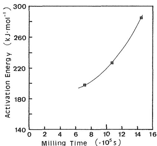
Fig. 4 Activation energy for crystallization of Ni<sub>50</sub>Ti<sub>50</sub> amorphous alloy prepared by mechanical alloying.
