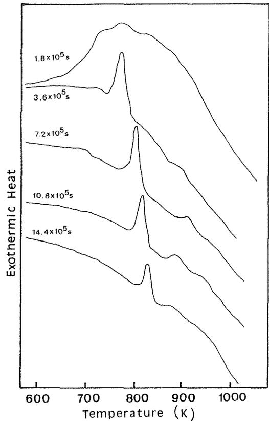
Fig.2 DTA curves (rate 0.6 K/s) of  $Ni_{50}Ti_{50}$  alloy produced by mechanical alloying.
