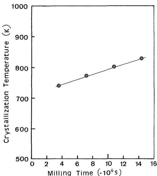
Fig. 3 Crystallization temperature of Ni<sub>60</sub>Ti<sub>50</sub> amorphous alloy produced by mechanical alloying.
