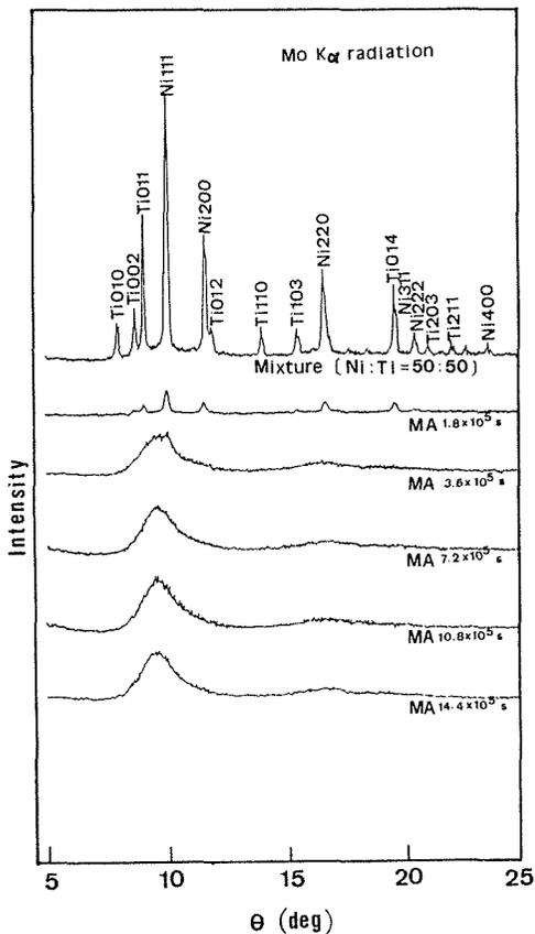
Fig.1 X-ray diffraction patterns of  $Ni_{50}Ti_{50}$  alloy produced by mechanical alloying as a function of milling time.
