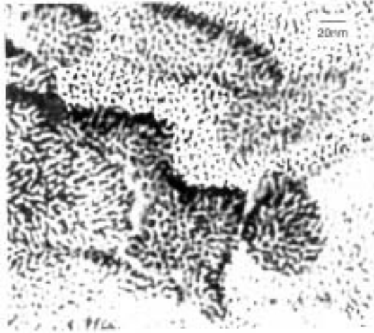
Fig. 11 TEM image of the mixed film of Pc and Cu by simultaneous vacuum deposition method. Nano-clusters and nano-rod around the cluster were observed.
