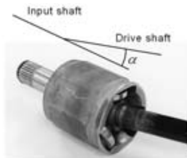
Fig. 1 Tripod constant velocity joint and its inner structure
